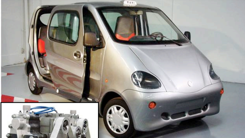
Next year, is powered entirely by a tank filled with compressed air.
